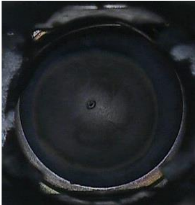
Failed IPF Beam Window
